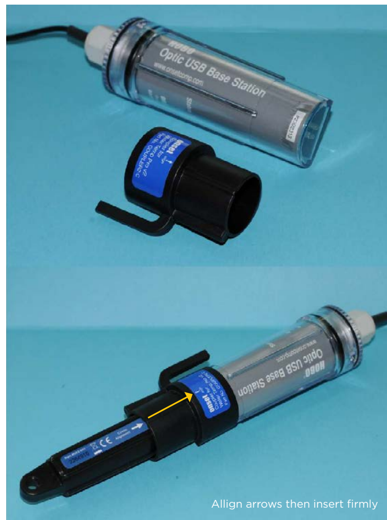
Figure 4.2: Optic base and coupler used for HOBO-U22 data logger launching and offloading.
